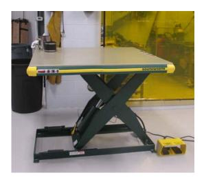
**After:** Raises equipment to reduce bending and reaching
