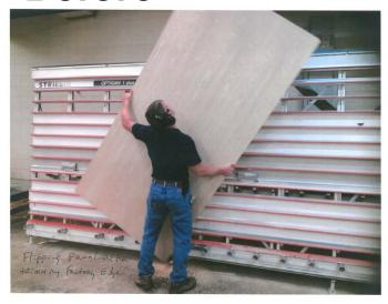
**Before:** "On our current saw the cabinet makers are required to lift a sheet of plywood (48x96 or larger) from a rack.."
