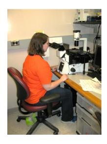
After: Raised and angled eyepiece to reduce bending
